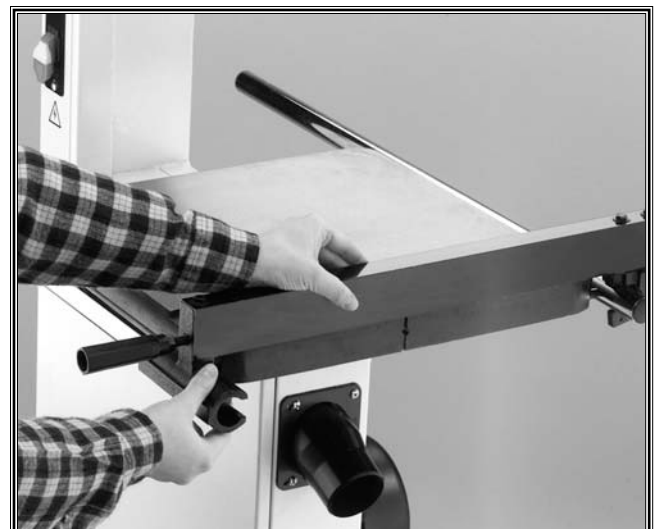
Figure 23. Starting fence on rail.
